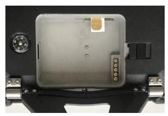
Figure 2: Inserting the USIM card
