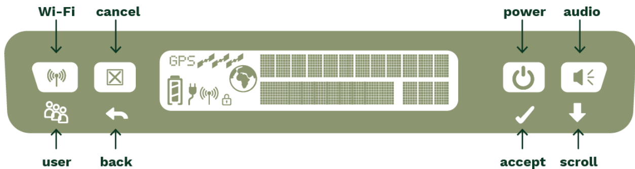
Figure 5: Layout of the LCD and keypad
