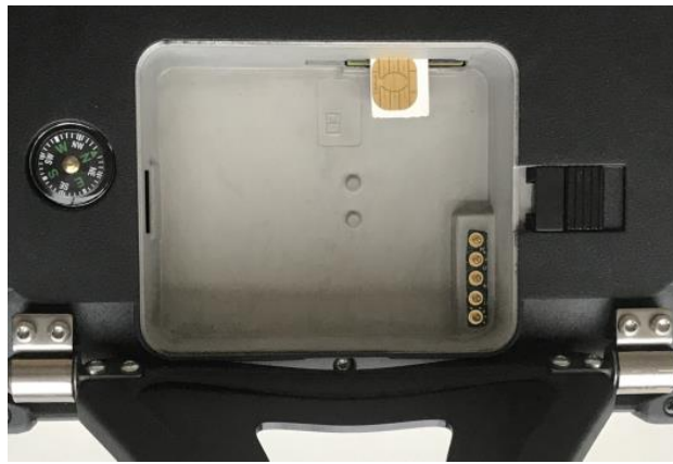
Figure 2: Inserting the USIM card
